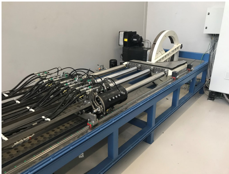
Figure 29: The CorPower dynamic seal test rig.
