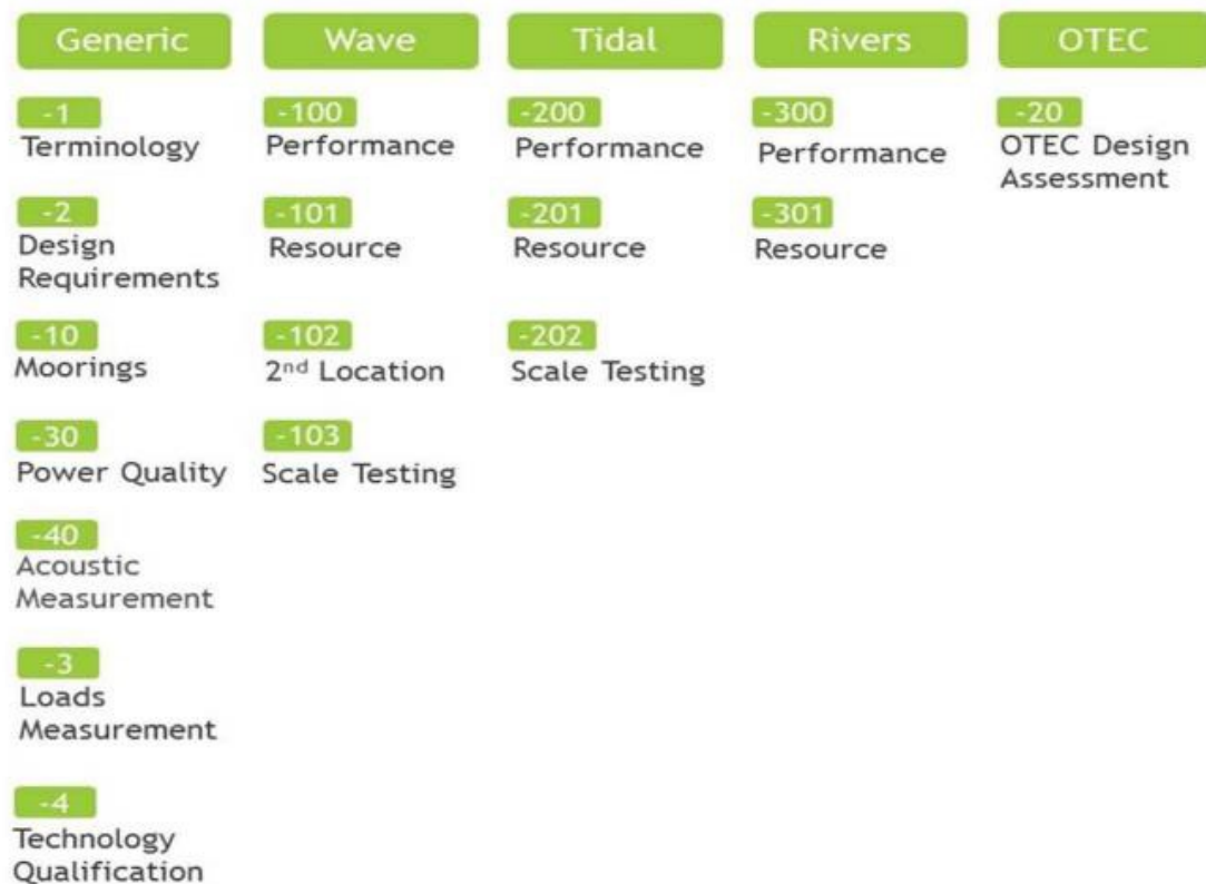
Figure 1: Overview of IEC TC 114 62600 series of standards for marine and water current energy converters.
