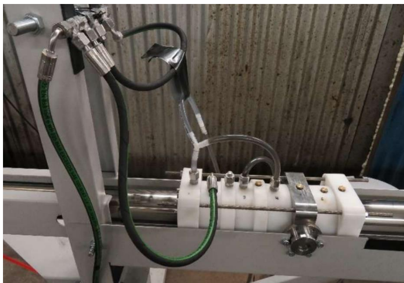
Figure 36: Seal block used by Wavepiston until now to test seals.
