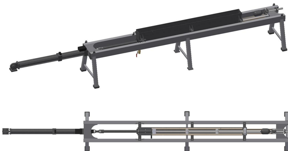
Figure 38: 3D sketch of the full-scale pump test rig.
