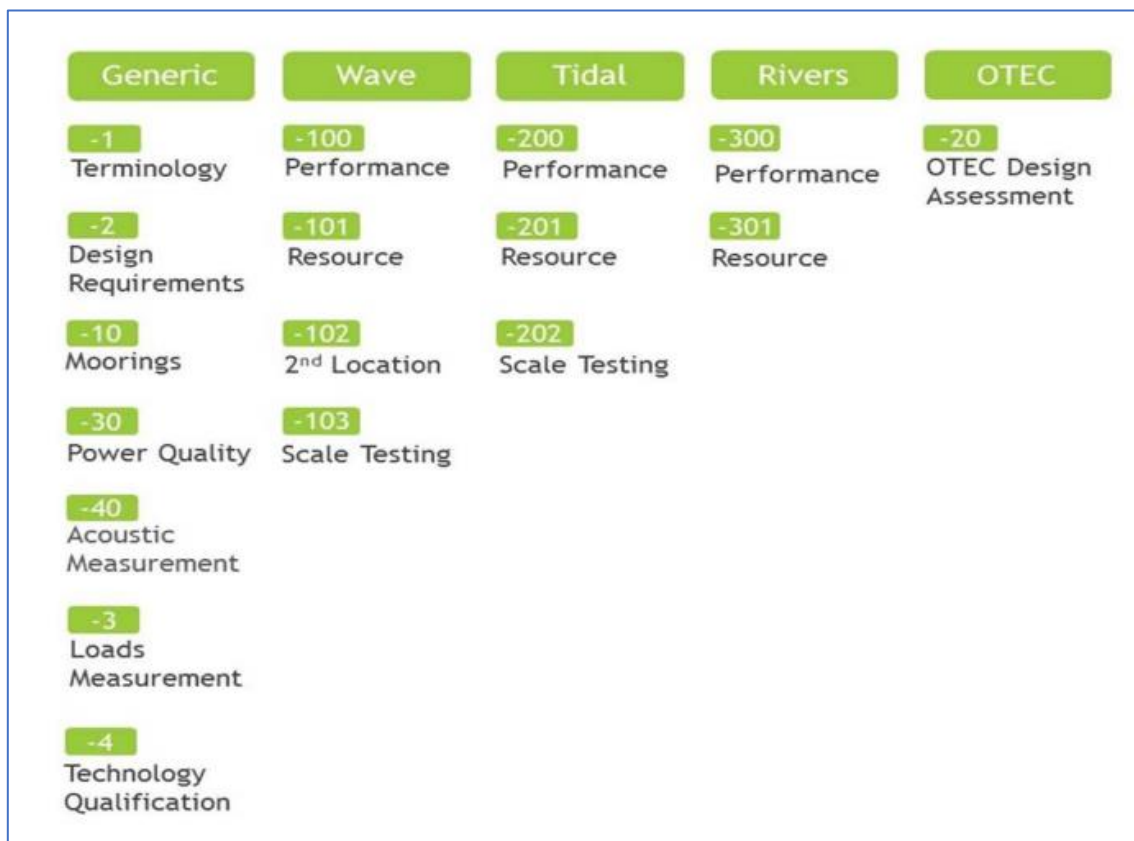
Figure 26: Overview of IEC TC 114 62600 series of standards for marine and water current energy converters [49]
